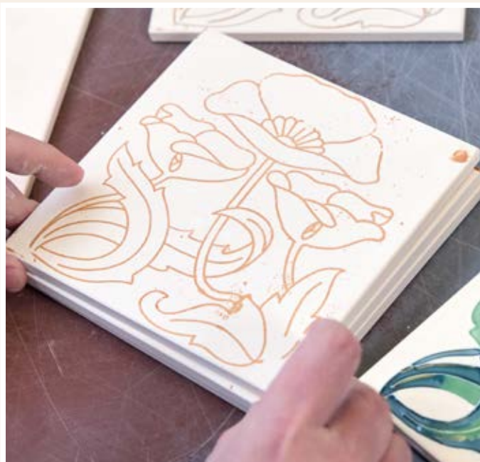
▲ The pattern is stenciled onto the blank tile biscuit.
