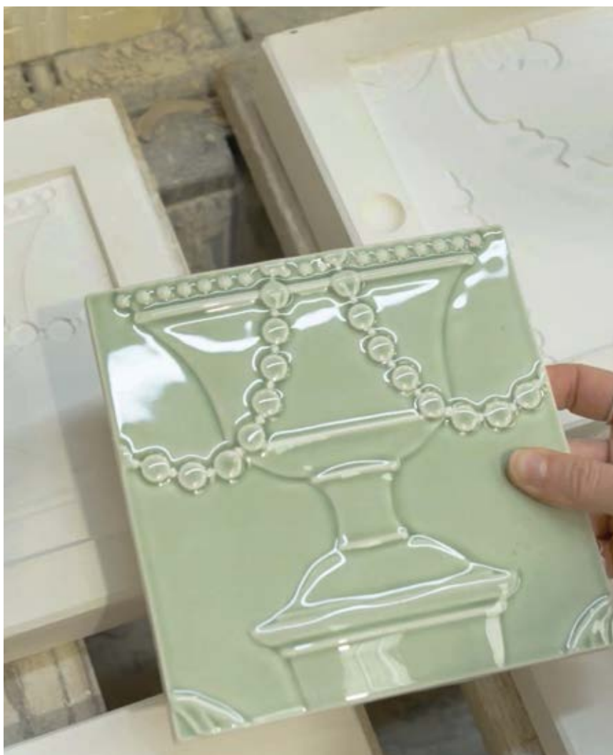
▲ Bespoke glazed moulding with plaster moulds
